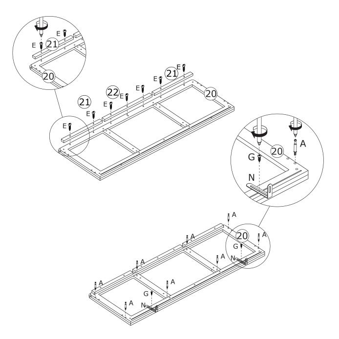
Screw eccentric rod(A) into board 20 and fix part(N) with screw(G) as shown.
