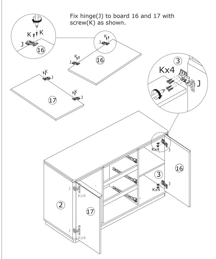
Assemble door 16 and 17 to board 3 and 2 by fixing hinge with screw(K) as shown.
