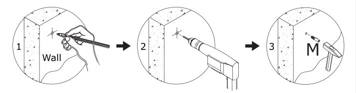
Install anti-tipping device as shown.
