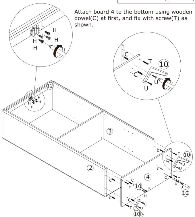
Attach leg 10 to board 4 using wooden dowel(C), and fix with screw(U) as shown.
