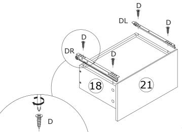
Fix runner(DL) and (DR) to plate 17 and 18 respectively using screw(D) as shown.
