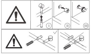
Connect the two components(assembled in step 3 and 6), put cam lock(B) into plate #25,#26, and turn clockwise to tighten as shown.
