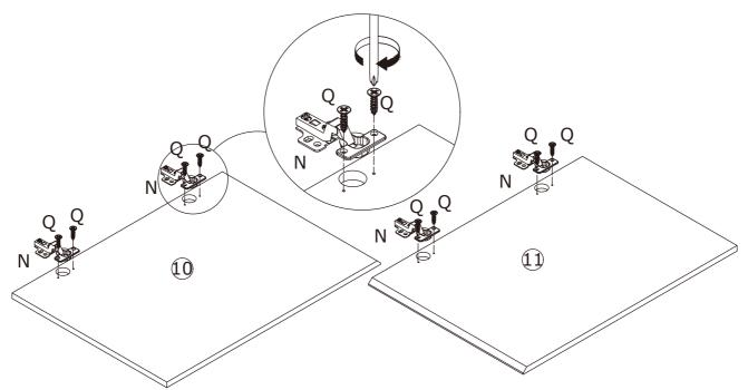
Please don't use an electric drill or use force to rotate, may cause crack.
