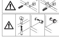
Put cam lock(C) into holes in plate 5,6,4,3 and turn clockwise to tighten as shown.
