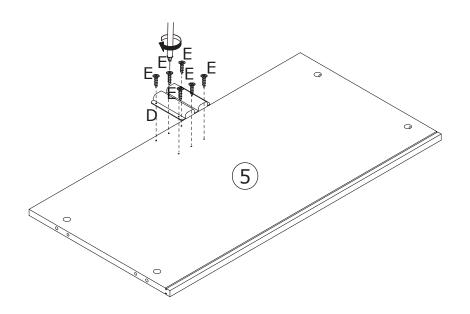
Fix part(D) to plate 5 using screw(E) as shown.
