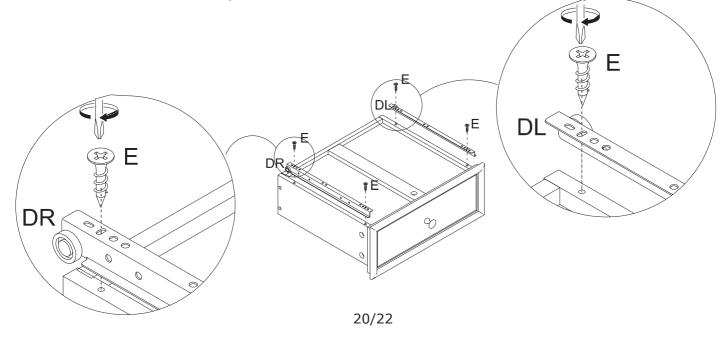
Align the assembled drawer with the guide wheel according to the serial number and put it into the cabinet in turn, as shown in the figure
