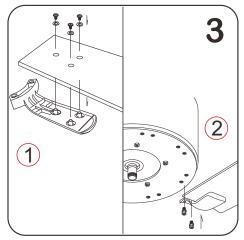
1.Match the fan blade hole to the According to the different installation fork and lock the screw as shown in the figure. 2. Then align the fork with the hole in the motor connecting plate and lock the screw to ensure that the screw is firm.
