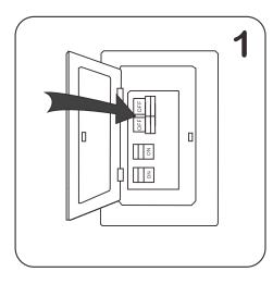
Turn OFF the electrical power at the main fuse of circuit breaker.
