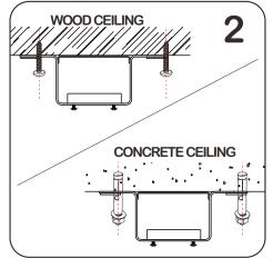
ceiling, select the corresponding installation screw for installation
