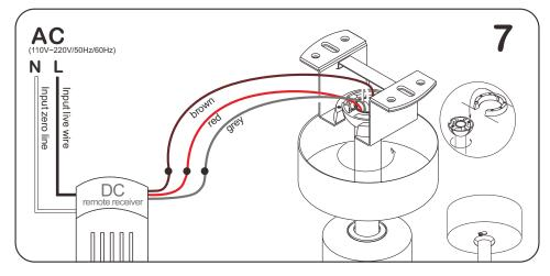
After hanging the fan suspender into the hanger, rotate and clip it into the groove, then connect the wires according to the color, and finally put on the hanging cup. After rotating the hanging cup, lock the hanging cup screw
