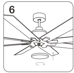
Screw the decorative cover clockwise into the motor shaft as shown in the figure, and make sure it is firm.
