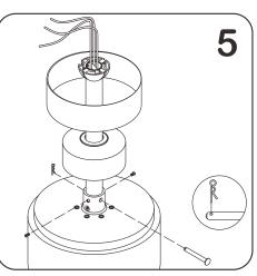
Clip the suspender into the fan motor, then rotate it to align with the hole, insert the cross bolt screw, lock the R pin, and finally lock the two screws on the hanger head.
