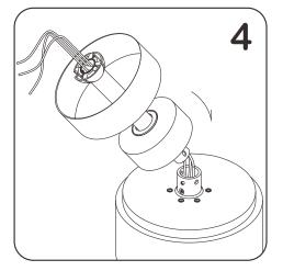
According to the figure, put the suspender into the upper cup, decorate the cover, and then thread the motor wire.
