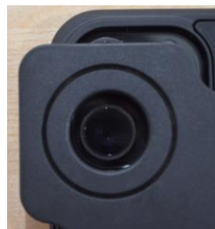
Figure 5 – Concentric alignment of the magnetic tab cutout with the desired camera lens
