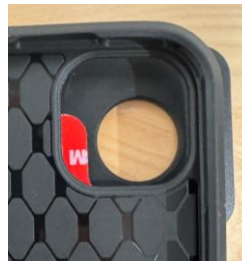
Figure 3 – Excess adhesive tab extending beyond the phone case camera cutout
