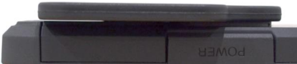
Figure 2 – Magnetic Tab placed flat on the back of the phone case. Notice the clearance between the phone case protrusions around the camera lenses and the back face of the magnetic tab.
