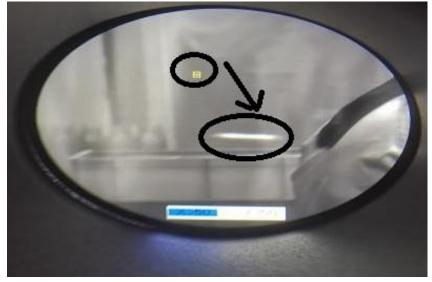
Above, the yellow aiming box isn't over the white flashing beam, in this case it needs to be moved down and right.
