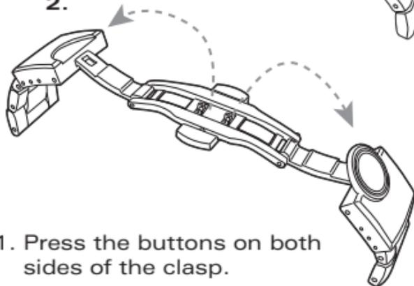
1. Press the buttons on both sides of the clasp.
