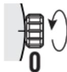
1. Unscrew the crown by turning it anti-clockwise.
