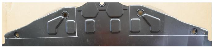
Re-install each Quarter Guard with the stock forward (2x) T-40 Torx bolts. Leaving the countersunk mounting holes empty for now.
