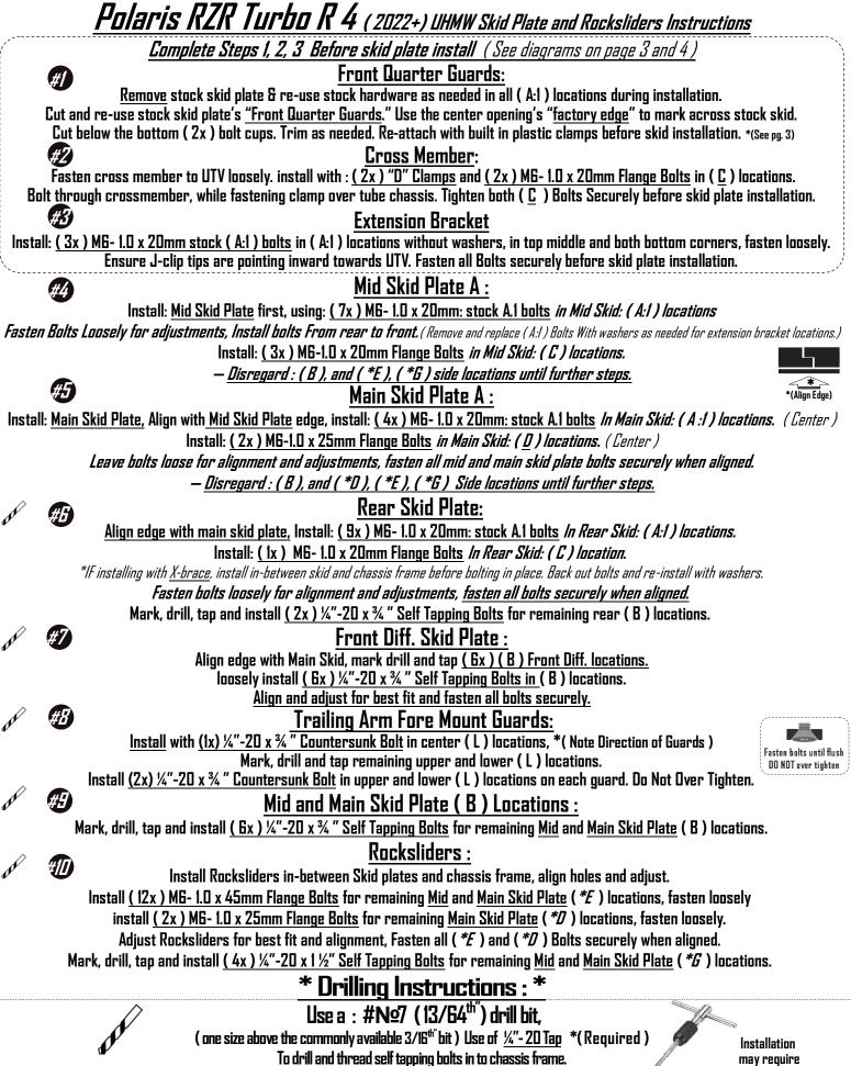
Finger Thread All Bolts Prior To Fastening Securely With Power Tools.
