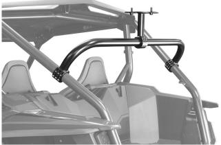
Designed to mount holding Wheel in 3 locations: Fastened securely on Center post mount, With tire resting Snug on pole on both sides to avoid vibration
