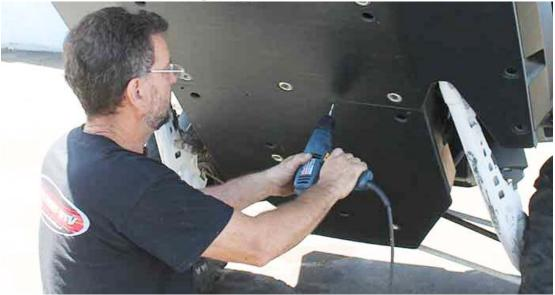
**10. Mark Rock Slider holes and drill pilot holes using 3/16 bit. Install new bolts and washers.**
