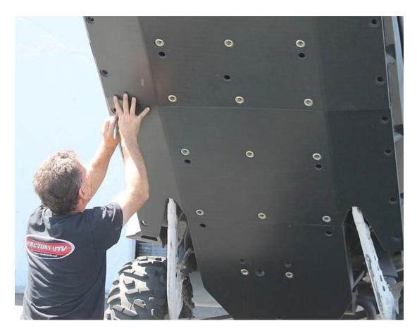
**11. Tighten all hardware up securely. (Loctite recommended)**
