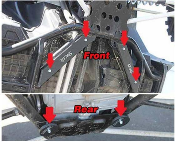
**3.** install front main skid to allow slight movement, with center bolts using stock hardware
