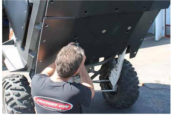
6. Install rear skid plate \*Forward skid plates always overlap rear skid plates.
