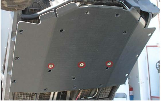
4. While pressing skid against spacer to hold it in place, remove bolts and reinstall with washers.
