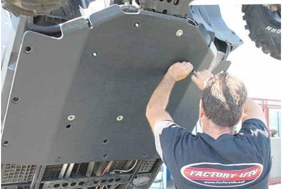
5. Install Center skid plate to allow slight movement. \*Forward skid plates always overlap rear skid plates.
