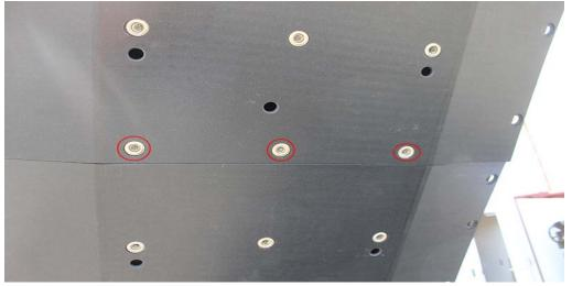
**9. Drill 3/16 holes and install countersunk bolts in front side of Rear skid plate.**
