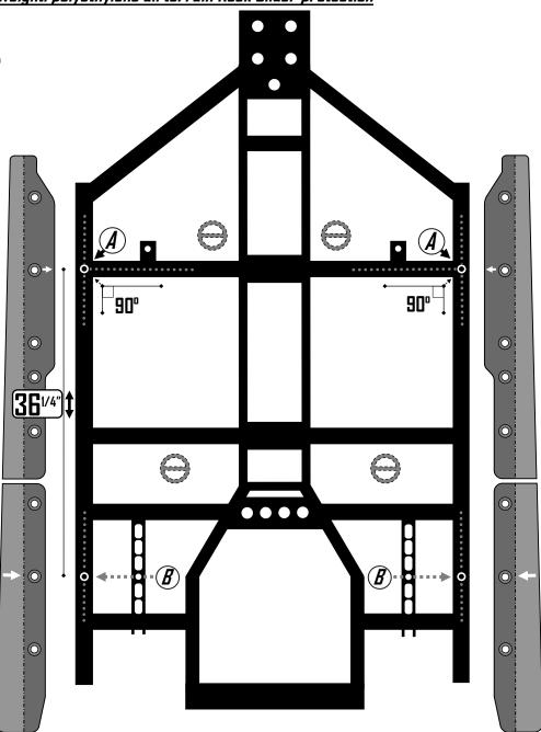
Ensure each mounting hole is drilled in to the center of the "Round" chassis tubing.
