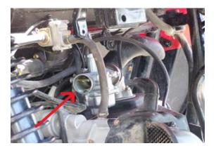
5. Install new intake tube to carb using supplied rubber hose section and hose clamps
