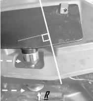
After Brackets are installed, Re-install Skid plate
