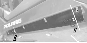
Use spacers to align bracket until mount is flush with stock plastic
