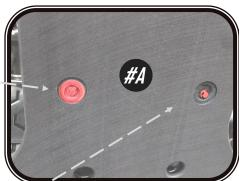
For the mounting holes under the UMHW spacers, back out one bolt at a time, ( in 2 steps) so it doesn't slip out of place
