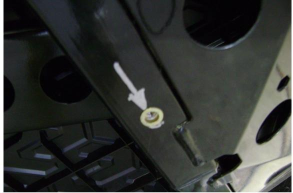
4. Hold up either skid plate and line up rear 4 holes with the nutserts.
