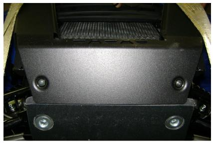
2. Finger tighten front 6 holes using 6mm x 35mm bolts.
