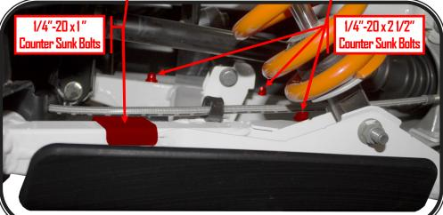
(4x) 1"x 1" D Clamps (4x) 1/4"-20 x 1" Counter Sunk Bolts (4x) 1/4"-20 x 1 1/2" Counter Sunk Bolts (8x) Ny-Lock Nuts (8x) 1/4" Gold Washers
