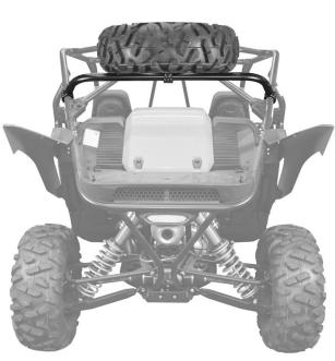
Designed to mount holding Wheel in 3 locations: Fastened securely on Center post mount, With tire resting Snug on pole on both sides to avoid vibration
