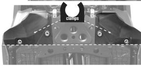
Cut and re-use stock skid plate "front quarter guards" Use the center opening's "factory edge" to mark across stock skid below bottom (2x) bolt cups. Cut as needed. Re-attach with built in plastic clamps before skid installation skid plate utilizes same bolt locations.
