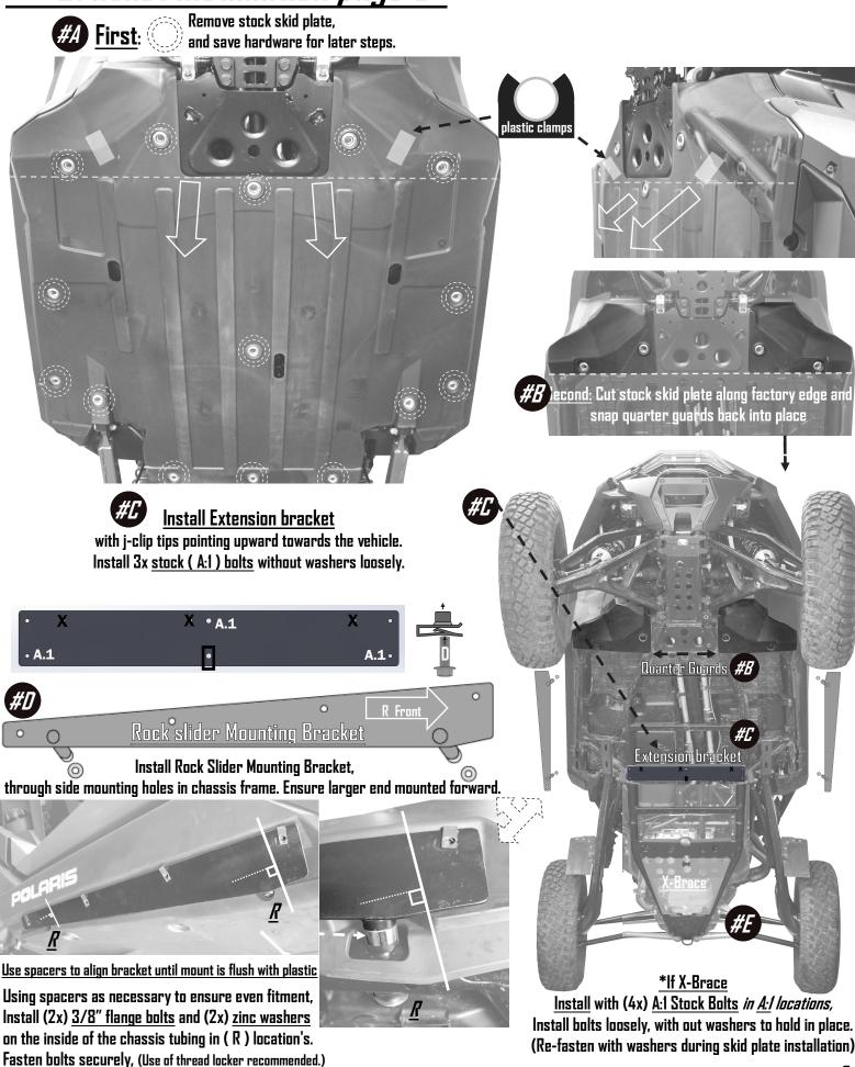
RZRTRSkd-Sldr — Factory UTV LLC ©2022 — Polaris RZR Turbo R (2022+) UHMW Skid Plate and Rock Sliders Instructions  $v_{3.5}$  pg. 3
