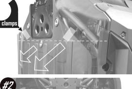
Second: Cut stock skid plate along factory edge, Remove remaining skid plates, save all hardware
