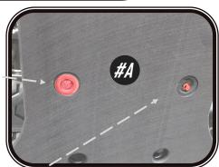
For the mounting holes under the UMHW spacers, back out one bolt at a time, ( in 2 steps) so it doesn't slip out of place Re-install bolt with washer
