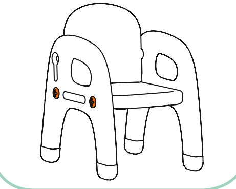
Insert the second chair leg (side) into the backrest/seat, as shown above and push tightly until the side is firmly in place. Place the chair in the upright position and insert the plugs as shown. Tighten the plugs with the included tightening tool or a coin.
