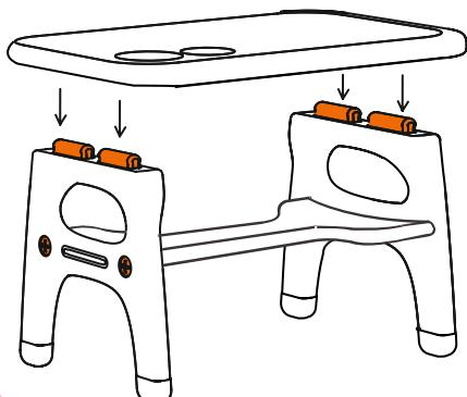
Connect the second table leg the same way and tighten the plugs, as done earlier. Align the recessed side of the tabletop with the table legs and press firmly until the tabletop is tightly held in place.
