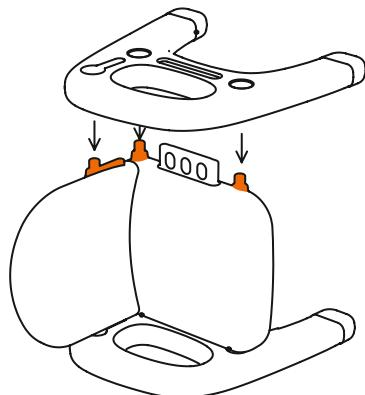
Place a chair leg (side) flat on the ground, insert the chair back support and seat into the holes of the chairside. Press firmly to secure the parts together.
