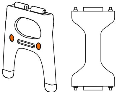
Position one side of the table legs as shown. Insert the end of the table shelf on one side. Install the included plugs on the table legs. Tighten the plugs with the included driver tool or a large coin.
