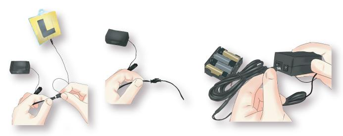
3.) Connect the inverter cable to the electroluminescent panel and ensure they are secured and connected.
