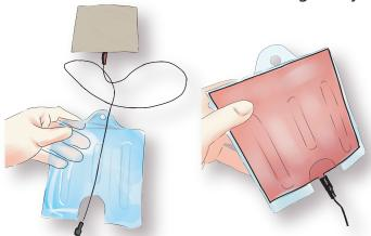
1.) Insert the cord of the electroluminescent panel into the bottom cut out of the transparent sleeve. Ensure the lighting area (pink side) is facing forward.
