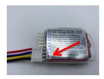
Notice the **(-)** on the bottom of the image. The **black wire** of the balancing tap (on the battery pack) will plug into the aligning prong; with the remainder following in sequence. Once plugged in correctly, there will be a repetitive alarm from the two speakers on the top of the unit. Return to the front view to see the voltage readings start to display on the digital screen. This cycle will go through the entire voltage reading on the battery pack, as well as the individual cell voltages.
