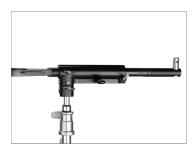
• Press the locking lever of the Docking Plate to remove the 54mm ring.
