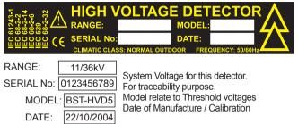
CLIMATIC CLASS: Normal. The detector will perform correctly over the temperature range -25°C to +55°C and in 20% to 96% humidity.
