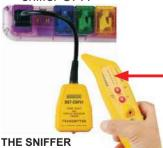
The Bar-Graph shows that the sniffer can detect the cable which is plugged into the socket. That mean that the transmitter is sending the signal and that sniffer can receive it.
