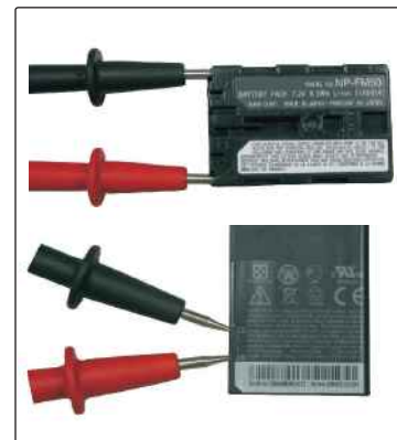
Li-ion Battery Measurement
