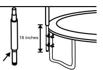
3. The set comes with 2 clamps per pole. One being attached 2" below frame, while the other being attached 2" above the end of the lower pole.
