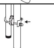
6. Now you can have the upper part of the pole inserted into the lower part that is already attached to the leg.
