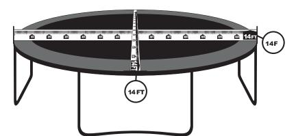
Measure your frame from one outside edge vertically and horizontally to the other outside edge so you get the correct measurements.
