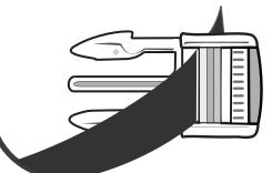
Turn the tie back and thread the end back through the clip, through the right slot this time
