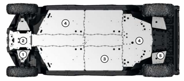
For ultimate durability and strength, all our Aluminum Skid Plates are made with High Strength 5052 H32 Aluminum <sup>3</sup>/16" (4.5 mm) thick.
