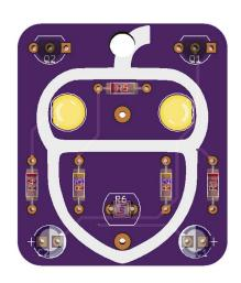
Align flat side of LED with the flat side of the part outline.
