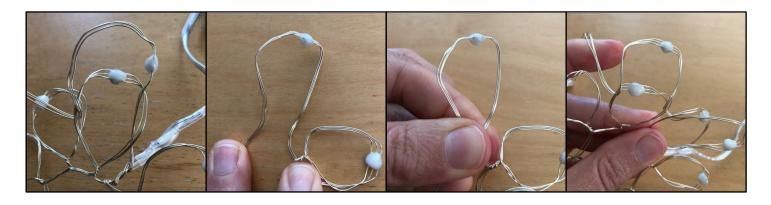
Keep pulling LEDs through loops, and as you go, turn the LED on the strand so that the rounder more translucent "top" is facing out. The Blob will eventually start to form a tube shape. You may need to bend each "stitch" inward as you go, to prevent the previous one from popping out (or in knitting parlance, "dropping stitches"). You'll figure out what kind of bends work for you as you go!
