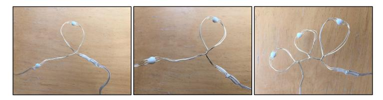
Bend the loop in a circle, and wrap the wire going to the USB connector to fix the circle.
