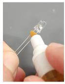
Place the component through the board, and make sure it's sitting flush or as close to the board as possible. Direction matters with some components like LEDs, read the instructions for your kit!
