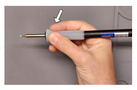
Wipe off the tip with brass wool using a firm backwards pull, repeat 2-3 times. There should be no chunks of solder on the tip, and the tip should be shiny.
