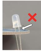
Turn the board over. On some components, you can bend the legs about 45°, to keep them from falling out.
