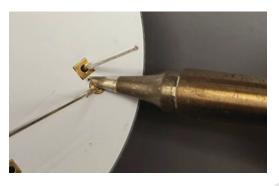
13 Touch the solder to the tip of the soldering iron, as close as you can to where the tip, pad, and component meet. Feed solder in as it melts, it should flow to the pad and around the component legs.
