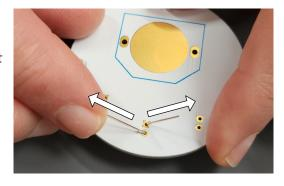
7 Rotate the board so that the component is at a comfortable angle to your soldering hand. You may want to tape the board down to the table to keep it from moving while you're soldering.
