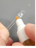
Place the component through the board, and make sure it's sitting flush or as close to the board as possible. Direction matters with some components like LEDs, read the instructions for your kit!
