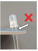
6 Turn the board over. On some components, you can bend the legs about 45°, to keep them from falling out.
