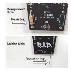
4 Paint a small amount of flux on the pads for the component you are about to solder. For throughhole components, you can also flux the leads where they'll contact the board.
