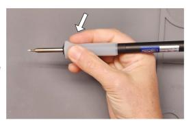
9 Wipe off the tip with brass wool using a firm backwards pull, repeat 2-3 times. There should be no chunks of solder on the tip, and the tip should be shiny.
