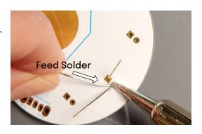
14 Pull the solder away, then remove the iron.
