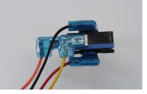
Place the LED into the LED holder, and make a note of which leg the flat side/cathode of the LED is contacting. You'll need to know this later when connecting the button to your project.
