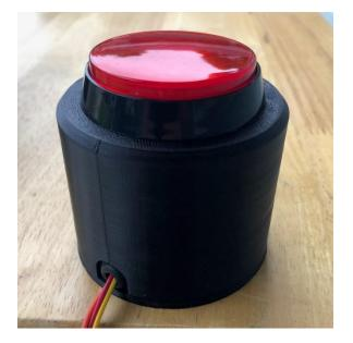
Note you will likely need to also print the nut tool in order to screw the nut on. The hardware in the kit allows you to attach the lid to the main enclosure body. The grommet protects the wires from abrasion – you will have to cut the grommet in order to put it around the cable.
