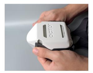
**Step 5** Finally, push down the bracket area on both sides of its upper section.
