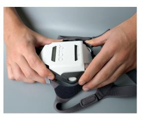
**Step 4**Push one and then the other clip into the openings until the bracket surface is flat against the ORM, and then tilt down
