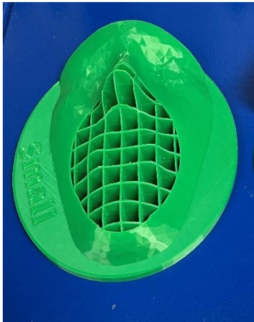
1. Printed Adult Small Face Form ISO # 16900-5- 2016 2. Mask Under Test
