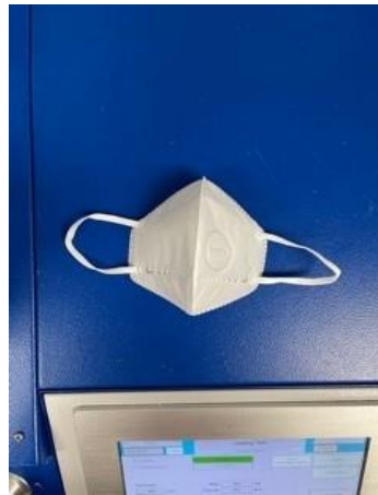
1. Printed Adult Small Face Form ISO # 16900-5- 2016 2. Mask Under Test
