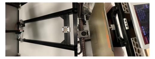
The pin mount was hitting the deflanged GT20 in the z-stop; requiring moving Z-stop away from extrusion by 2mms. This was accomplished by using longer screws using nut and 5mm washer. I will be replacing nut and 5mm washer in future with printed spacers.
