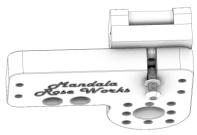
Insert the alignment key on the pin base into the slot on the yoke, and lightly secure it with a m3x10mm button head screw and m3 washer. Do not tighten down yet as you still have final alignment to complete.
