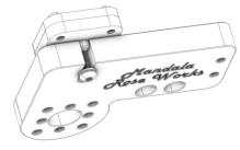
Insert the alignment key on the fixed mount base into the slot on the yoke, and lightly secure it with a m3x10mm button head screw and m3 washer. Do not tighten down yet as you have final alignment to complete.
