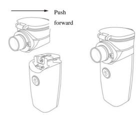
(2) Remove medication cup from device body. Press and hold the "PUSH" button on the body, and push medication cup away from the device body.
