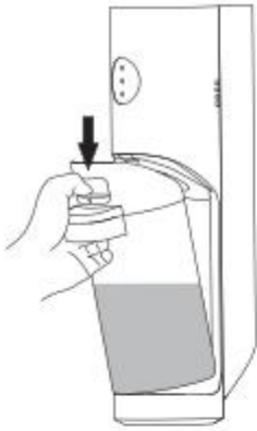
Remove the wastewater tank
