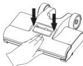
Press the upper cover of roller brush in the arrow direction until a "click" sound is heard, so the installation is completed
