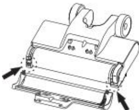
Insert the latch of upper cover of roller brush into the hole in the arrow direction
