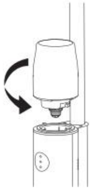
Remove the clean water tank
