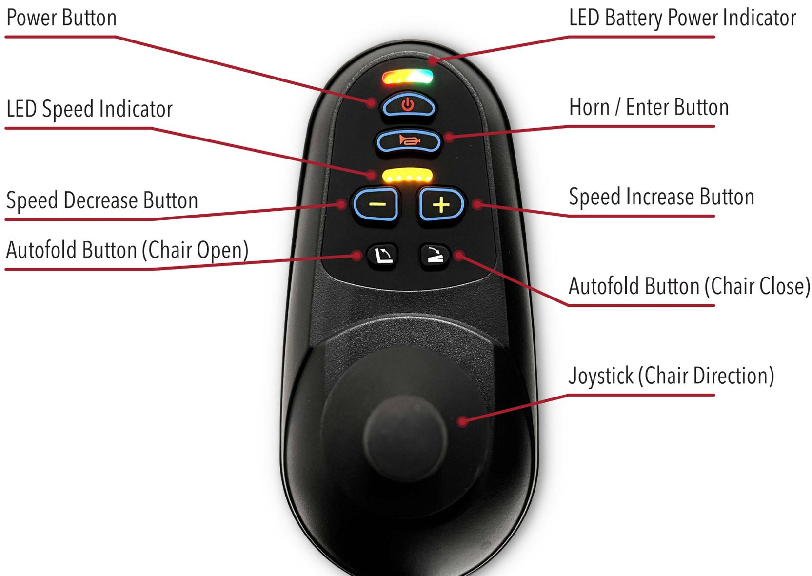
**Power Button:** To turn on the chair, press the power button. To turn it off, press the button again. When the chair is powered on, the LED Battery Power Indicator will light up.
