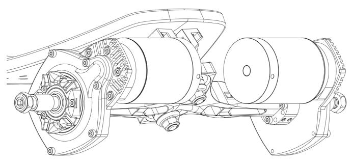
Wheels can be pushed onto the push fit adapters and wheel nuts tightened as normal. Wheel nuts should be tight enough to remove any sideways play in the wheel but not so tight as to add additional friction to the rotation. If your wheels have the correct bearing spacers inside you should be able to tighten the wheel nuts fully and then check that things still run smooth.
