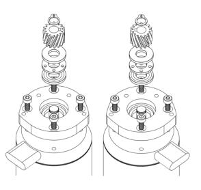
Apex JUMP DRIVE uses thrust bearings to reduce the strain on the motor bearings, for this reason it is important that the correct gear is installed on the correct side. Once built your motor assemblies should match those shown to the right. Double check this now.
