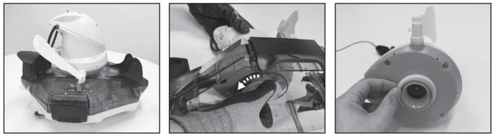
2. Use the screwdriver to unscrew the 4 screws located at the bottom of the head to release the bottom plate first. Then unscrew all the screws at the base as shown. Pry open the base to expose head inside.
